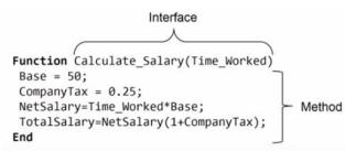
This is an example of a function. Its name is "calculate\_salary". It has one input : Time worked which reprensents the number of hours worked by an employee. The method then calculates the total salary taking into account the base salary per hour and the company tax.
