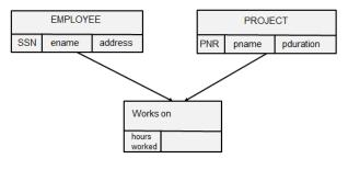
This relationship types has serious **implications** for data usage. Suppose we have a query that asks for all projects an employee is working on. To solve this query, we first need to select a set in a set type employee- works on. For each member, determine the owner in the set type project-works on. Go the other way around in case we need to find all employees working on a project. This is an example of procedural DML.
