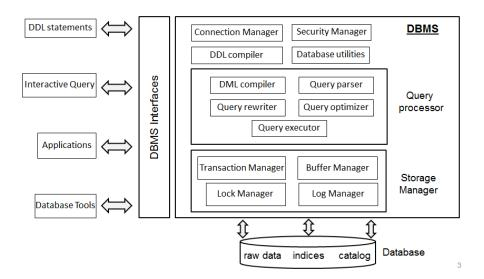
This is an overview of the key components of DBMS. This figure is by no means exhaustive! Some components may be left out, some others added.
