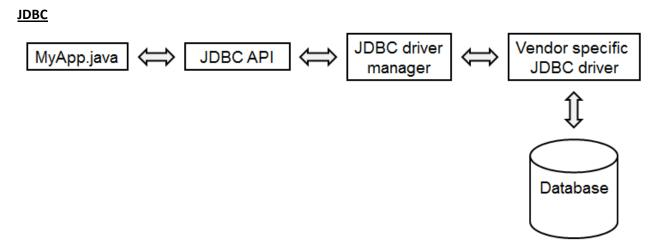
The file MyApp.java contains the java source code of the database application. He uses the JDBC API to call the JDBC driver manager wich will use the vendor-specific JDBC driver to communicate to the unerlying relational database. A key advantage of JDBC is that it provides a uniform access interface to verious underlying data sources. Given its popularity, many database vendors provide support for it such as Microsoft, Oracle, IBM, etc. It is also supported by MySQL.
