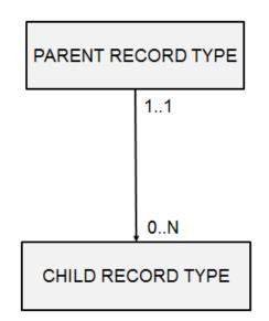
In this model, all record data needs to be retrieved by navigating from the root node of the hierarchical structure. In other words, the DML adopted is procedural, which is not so nice. It is also limited in terms of expressive power.
