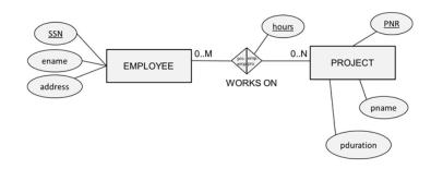
Here we can see the relation WORKS ON defined. It has 2 foreign keys: SSN and PNR which together make up the primary key and can thus not be null. The hours attribute type is also added.
