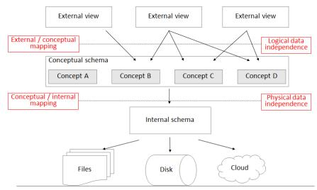
The three-schema architecture is an essential element of any database environment or application. This figure illustrates this architecture.
